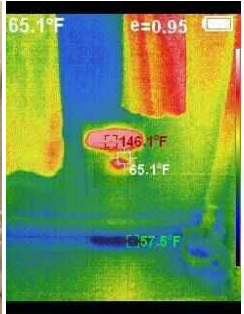
Thermal Image - Cadet Wall Heater (Representative Picture)
